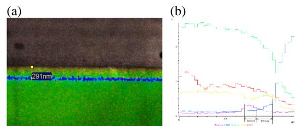
Fig. 2. SEM cross-section image of the sample with inset of EDS intensity of elements
