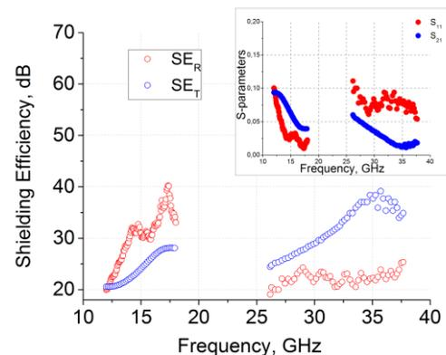
Fig. 1. Shielding efficiency and S-parameters (inset) of the 3D printed pyramidal samples in Ku- and Ka-bands
