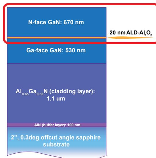
Figure 1. Schematics of N-face GaN grown on ALD-Al<sub>2</sub>O<sub>3</sub> to form a waveguiding structure with polarity inversion.
