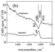
1 pav. (a) Image of a CNT/graphene system obtained at 1585 cm<sup>-1</sup>. Point #1 and point #2 have the same brightness while corresponding spectra (b) at resonance frequency show "peak" and "dip", respectively.
